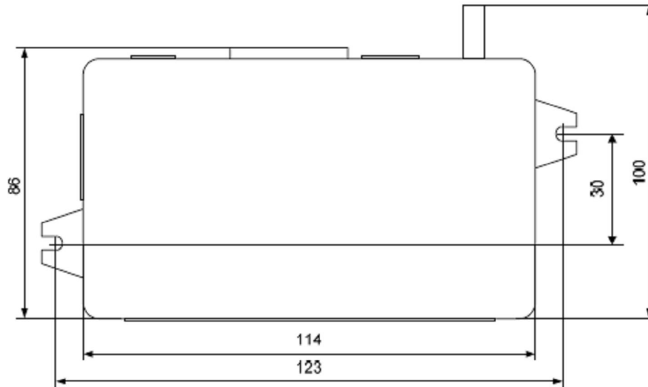
Figure 3. Dimensional and mounting specifications
